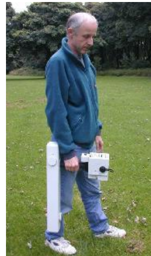
Figure 6. Geoscan Fluxgate Gradiometer (photo Geoscan Research website)
