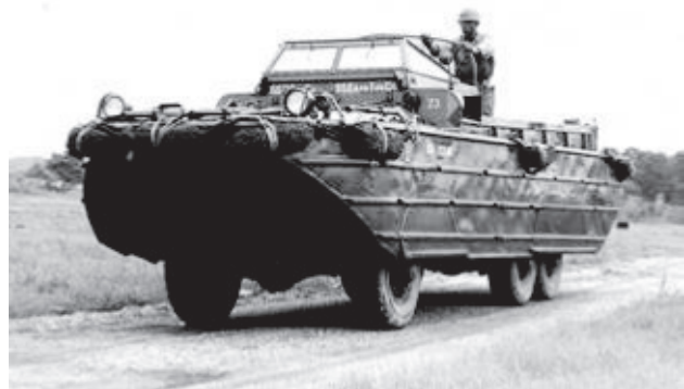
D (designed in 1940), U (utility), K (all-wheel drive), and W (dual rear axles)
