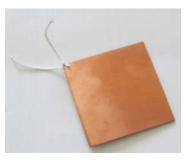
circuit reduced the Q to 100 at the same frequency after retuning the Q Meter. The piece of PCB has a self capacitance of 135pF which equates to approximately 20pF per square inch. This is an extreme example but does show that PCB losses must be taken into account, particularly in high impedance RF circuits, even at relatively low frequencies. You must therefore check the performance of your proposed circuit every time.
