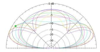
EZNEC can also provide plots of the horizontal radiation patterns of a given aerial on different bands (80m, 40m, 20m and 15m) as shown in the following picture. The increase in the number of lobes as the frequency is increased is clear:
