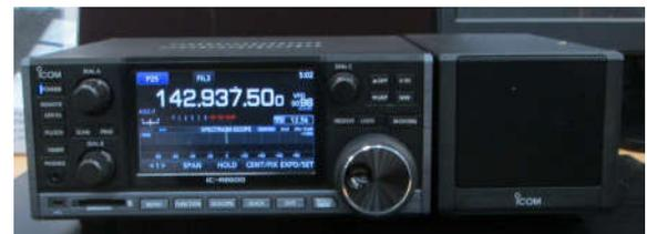
10KHz - 3GHz receiver excluding cellular allocations, AM/FM/SSB/CW and an internal data decoder. Requires a 12v DC PSU.
