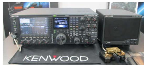
HF-50MHz transceiver, 200W, SSB/CW/AM/FM/FSK & PSK, Keyer.
