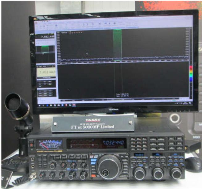
HF-50MHz transceiver, 200W, SSB/CW/AM/FM/RTTY & Packet, keyer, external display option.
