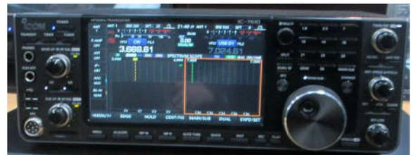
HF - 50MHz transceiver, SSB/CW/AM/FM/RTTY/PSK, DSP, 100W Tx, Spectrum Scope
