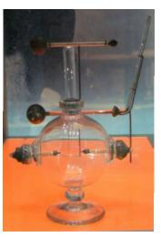
a spherical capacitor, consisting of a smaller sphere inside a larger one, with a gap between them that could be filled with air or anything else. Careful experiments with this device showed that electricity was not a weightless fluid and enabled him to measure the dialectic constant or permittivity of a substance.
