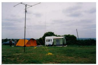
The beam is a G4MH two element three band reduced size yagi. Near the tent and caravan is a 33foot vertical for 40m plus our usual 264foot dipole supported on 45foot masts.
