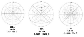
The dipole is aligned north south (page top to bottom) and as you can see, the pattern starts broadside (left to right) on the lowest frequency band and progressively changes to end fire (top to bottom) as the frequency increases. Impedance issues at the ATU can be mitigated by switching in different lengths of feeders.
