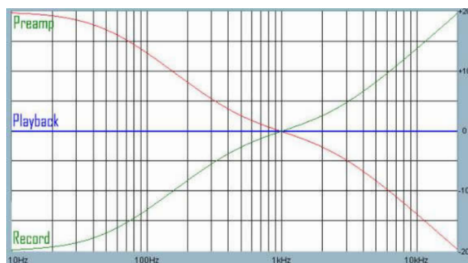
Fig.1 RIAA Curve Vertical Scale is in dB at 1 kHz
