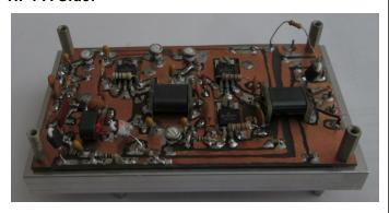
This is a three stage amplifier with negative feedback around each stage.
