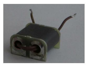
The gap between the copper areas can be clearly seen. The copper on the other end is continuous.
