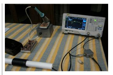
The display covered 1 - 206MHz with a sharp dip in SWR at 70MHz towards the left of the display.
