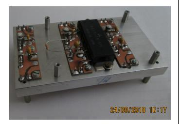
The fitted PA is for 144MHz and the empty spaces will hold the PAs for 432MHz and 70MHz, all by Mitsubishi.
