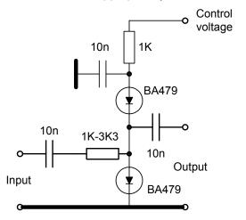
The circuit above may be used for AGC or ALC applications and will provide a typical attenuation range of 0-30dB depending on the control voltage. It has the advantage that the signal voltage across the diodes does not increase significantly once the attentuation action has commenced.
