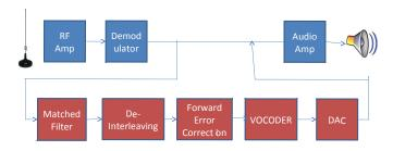
**Forward Error Correction:** is a mechanism for sending information using an error correcting code so that the receiver can make limited corrections in noisy or poor communication environments without requesting a resend.
