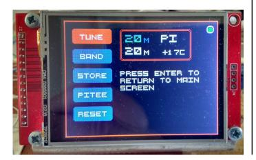
The prototype units are working and Alan is now designing in some protection functions, screening and general mechanics. The display unit screen views are shown below. The first one shows the operational screen containing an image representing the T or Pi in use, the band, transmit SWR and power.
