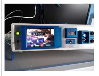
driven by DATV-Express software via homebrew ½ watt amp into his MOSFET amp suitably re-biased, thence via feeder to a Tonna beam pointing in my direction. Receive at both ends was a humble RTL T2 dongle via the Portsdown software. Screenshots direct from the Raspberry Pi 3.5" touchscreen.
