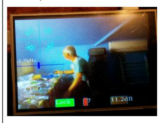
TX my end, BATC Portsdown with outboard amp then driving a Chinese '100 watt VHF' amp to 43dBm, feeder down garden to my fishing pole 12 element ZL special. At Martins end, ADALM PLUTO (upgraded firmware)
