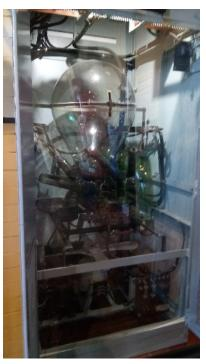
with glitches in the supply another excitation anode was provded with its own high voltage source.
