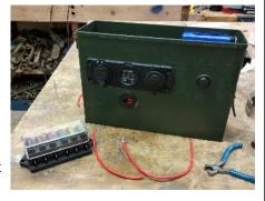
sockets, fuse board and switches.
