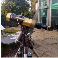
since this particular line is easily excited in Hydrogen. It is also invaluable for solar work such as watching sunspots and solar flares. Incidentally the box visible on the ground was part of the power/motor drive chain, since the tripod platform rotated very slowly to automatically track the Sun.
