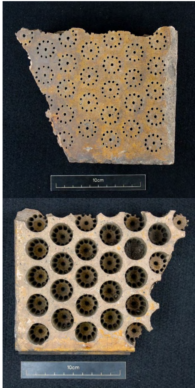
Plate 51 Malting brick from the Clementhorpe Maltings, York.
