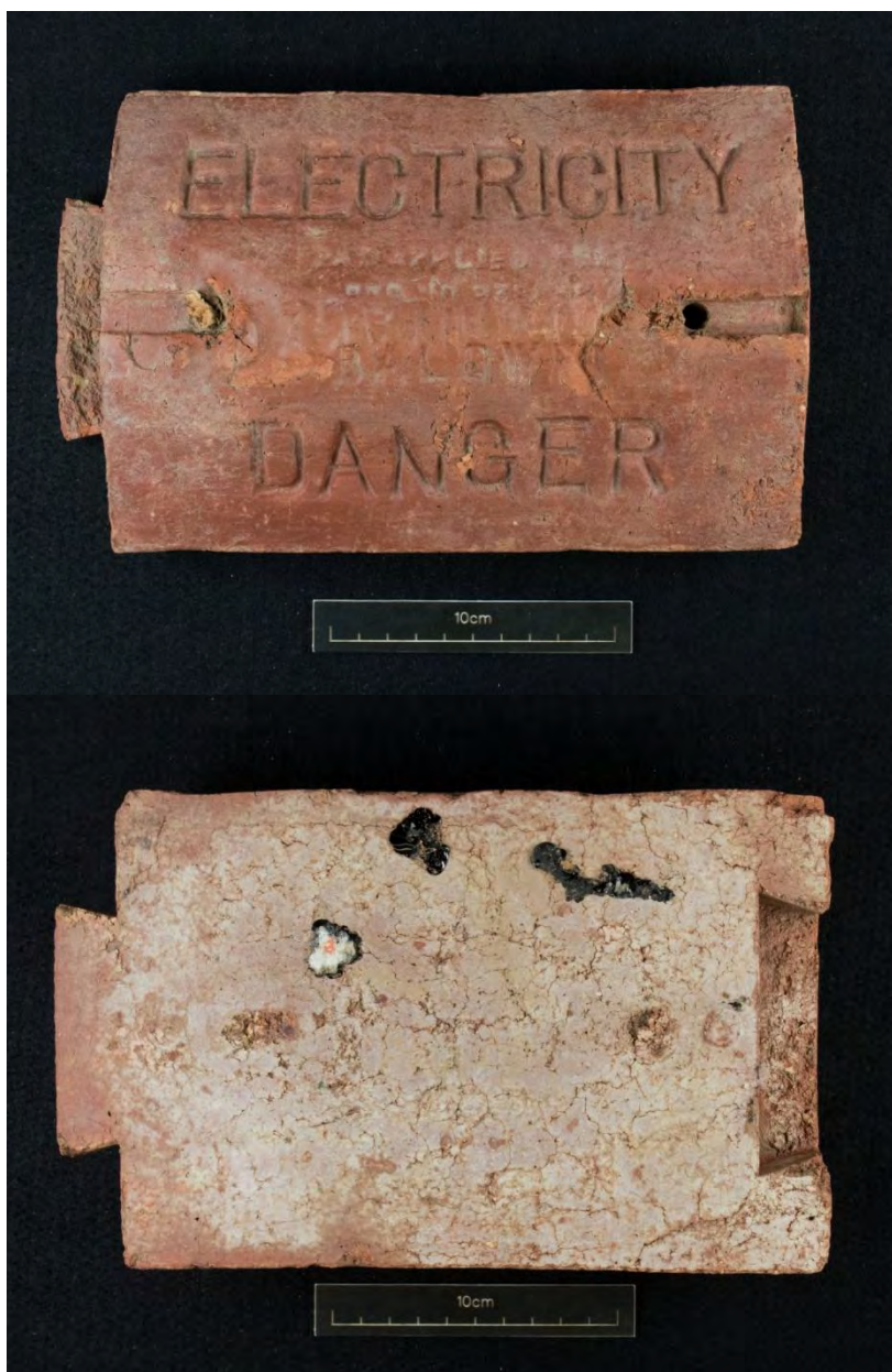
Plate 47 The upper and basal surfaces of a machine-made electricity duct. Form the Hungate excavations, York.
