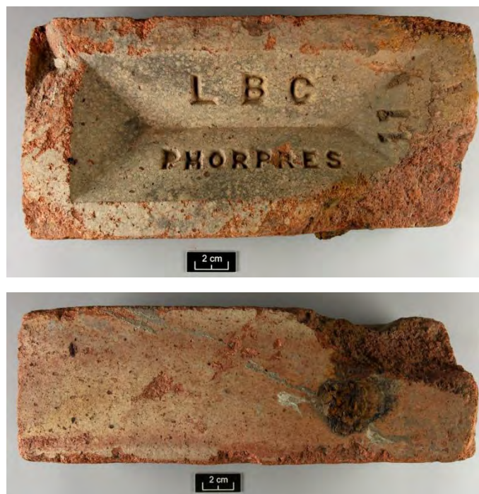
Plate 45 The upper bed and one stretcher of a modern brick from the St Leonard's Hospital excavations bearing the marker's stamp of the London Brick Company
