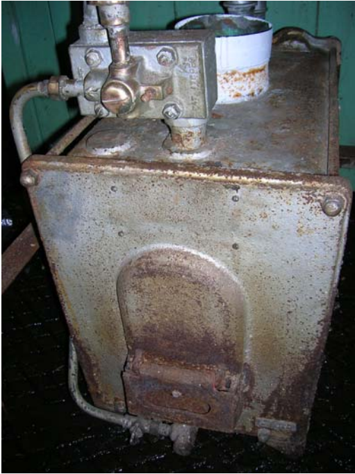
Photograph 41 – Before Conservation Rusty boiler
