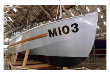
The picture above is taken from the starboard bow and shows the CMB with her wartime pennant number M103. Originally built to launch torpedoes (from a well at the stern as can be
