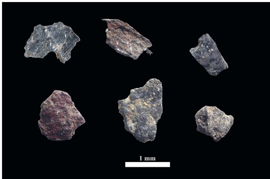
Fig4 Hammer scale flakes.
