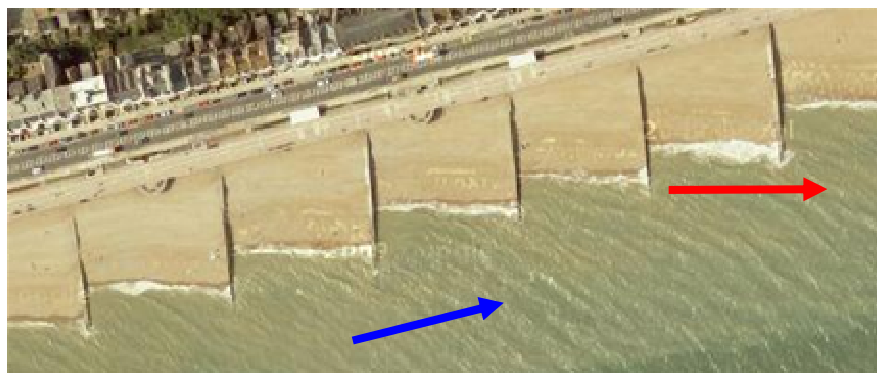
Fig. 12. Groynes. Also showing Longshore Drift (red arrow) and prevailing wind (blue arrow)
