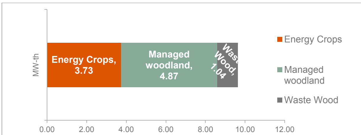
Figure 6-3. Technical potential for Biomass and Waste in terms of installed thermal capacity
