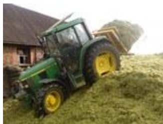
Alan uses a 'buckrake' to lift the wholecrop to the top of the pit
