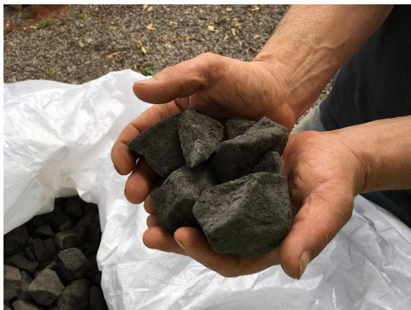
third picture. Then there is a 120mm, nearly 5", thickness of lime screed with the underfloor heating pipes sandwiched between these two layers. The stone floor is then above this. As I write this the glass insulating layer is being put in place, it is very light and looks and feels like clinker from a coal fire.
