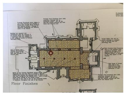
that will make up the finished floor. They are 30mm (a bit over an inch) thick. The original design had almost all of these tiles uniformly the same size but it was a requirement of the faculty approval by the Diocese that the random pattern of different sized tiles was created, with a uniform north-south line. You can see also that there is a darker
