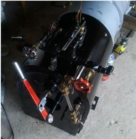
Figure 5 – The boiler fittings completed ready for inspection and testing.
