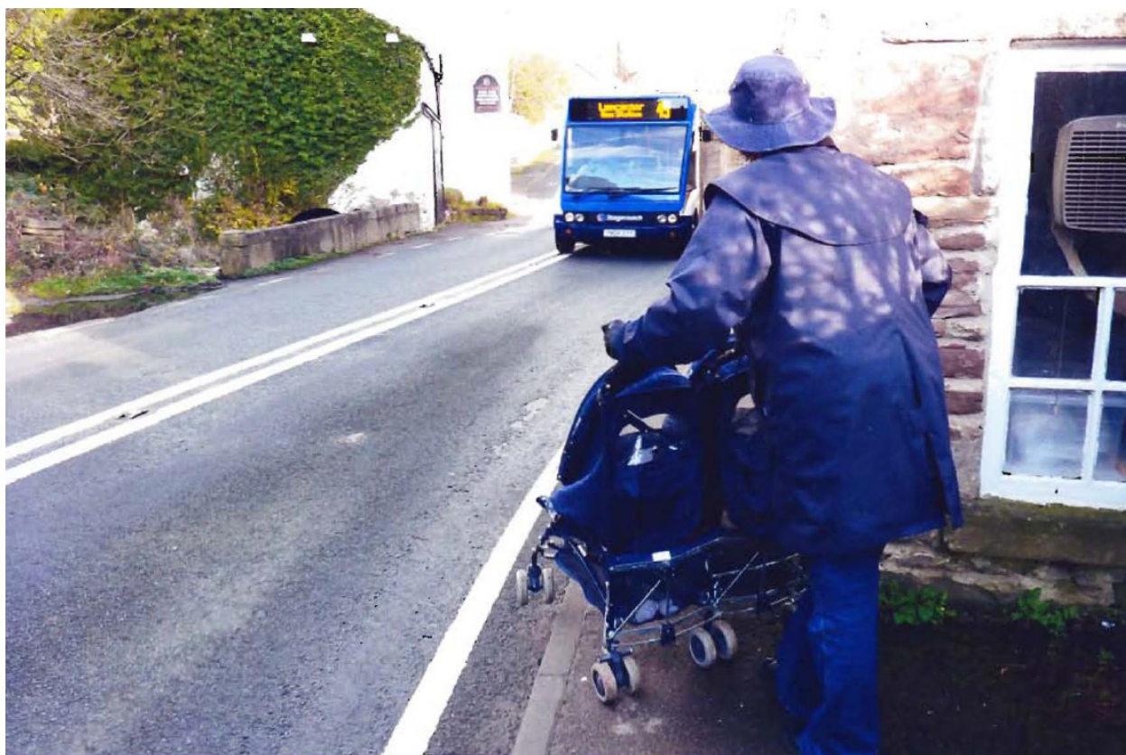
Figure 4 – Pedestrian having to enter the road on Church Brow as pavement width (68cm) is inadequate for pushchairs.
