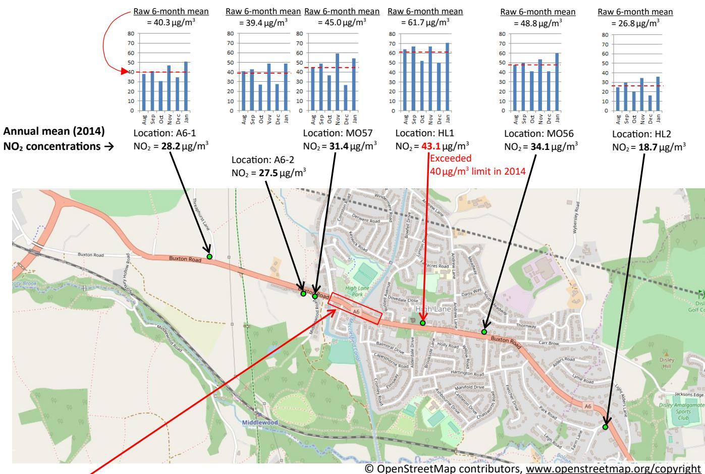
**Figure 1 — Measurements of NO<sub>2</sub> in High Lane in 2014.**
