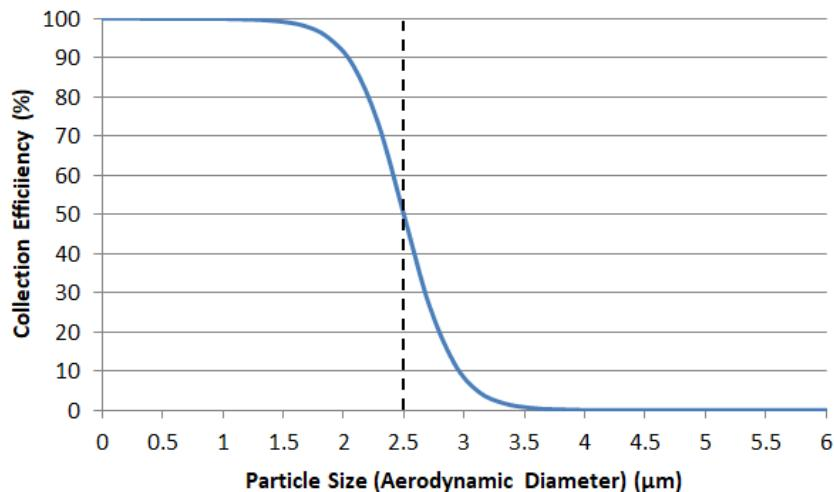
Figure 3 — Indicative Size-Selection Curve for a PM<sub>2.5</sub> Inlet
