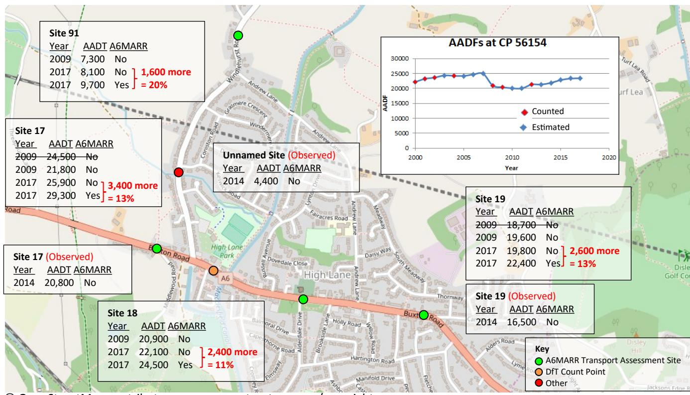
Figure 2 — Traffic Counts in High Lane in 2000-2017: Modelled and Observed
