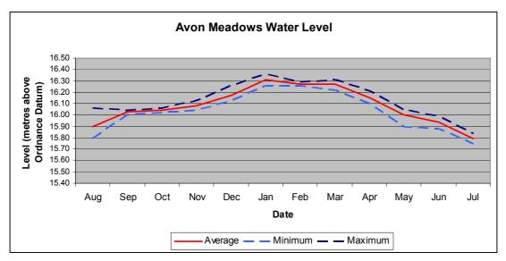
Note that the precise level at the top of the tilting weir is 16.36m and dry mud appears at the gauge board on the boardwalk at 15.48m.
