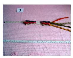
3. Fix the loose ends of one rope so that the two parts remain tightly together. In this case we have taped the red white and blue strands. Masking tape is good for this.
