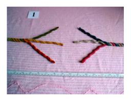
1. Separate the three component strands of each rope to be spliced. The length of the splice will be the length that you unravel – not twice as long!
