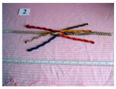
2. Push the two parts together with alternate strands from each rope. Pull them very close and tight together, otherwise the splice will be too soft and floppy in the middle.
