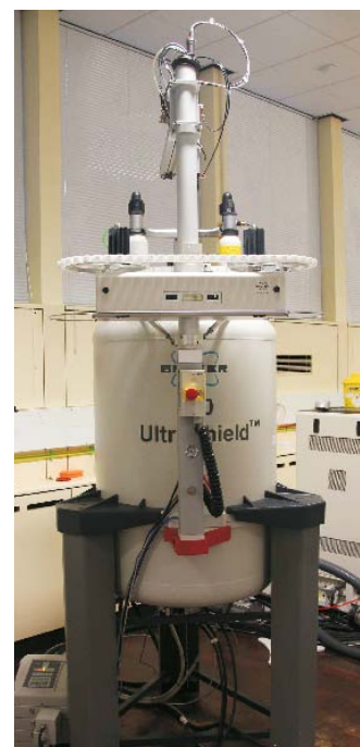
Nuclear Magnetic Resonance (NMR) spectrometer, used in the analysis of the composition of organic carbon.
