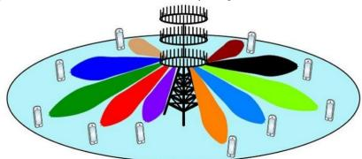
Standard MiMo networks tend to use two or four antennas. Massive MIMO, on the other hand, can have tens or even hundreds of antennas. For example, Huawei, ZTE, and Facebook have demonstrated Massive MiMo systems with as many as 96 to 128 antennas; Ericsson's AIR 6468, which the company claims is "the world's first 5G NR radio", uses 64 transmit and 64 receive antennas.
