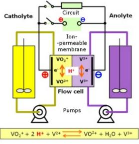
**Redox Flow Batteries** (Reduction/Oxidation) Unlike batteries where the reacting elements are held in, or form, the electrodes, in a Redox battery the charge is distributed throughout the liquids in a pair of cells, each with an electrode, either side of a membrane to prevent the contents mixing, but to permit charge flow between them.
