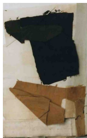
Two of Bancroft's four larger-sized fabric samples. The odd shape of each piece indicates the cuttings taken for testing. 6
