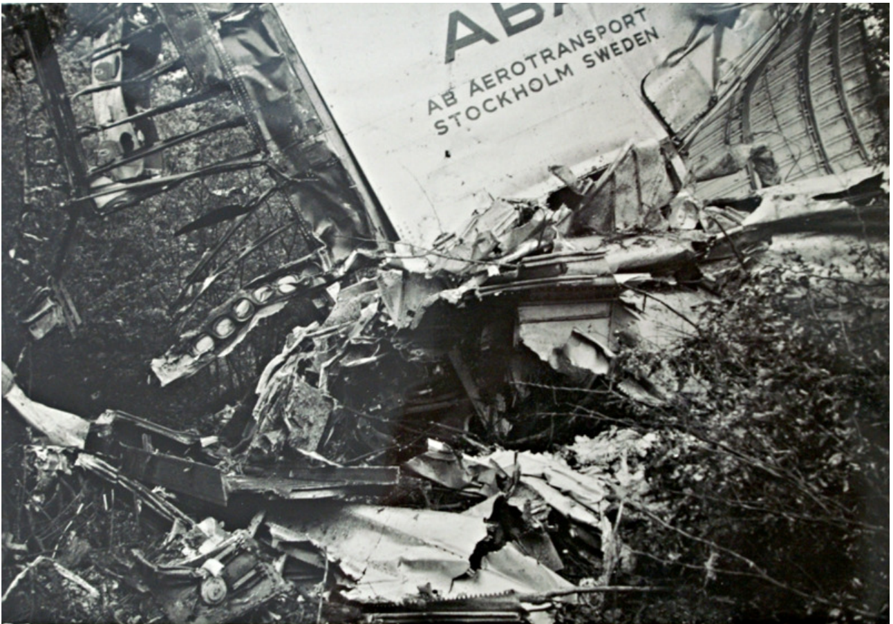
Fig. 2 - DC-6. Main wreckage remains of rear fuselage
